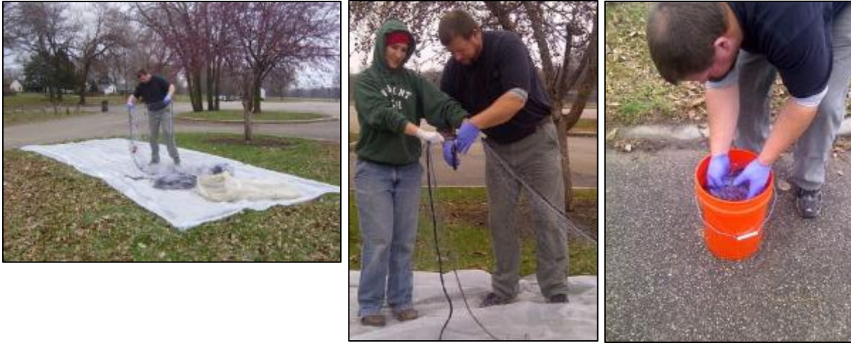
Figure 2.4.4. Net processing. Each net is laid out over a new plastic sheet, a middle portion (10 ft. or ~3.05 m) is cut away with sterile scissors, and the excised section is rinsed (with moderate swirling and dunking) in commercial distilled water in a new bucket for 1 minute in order to release DNA into bucket water for sampling.
