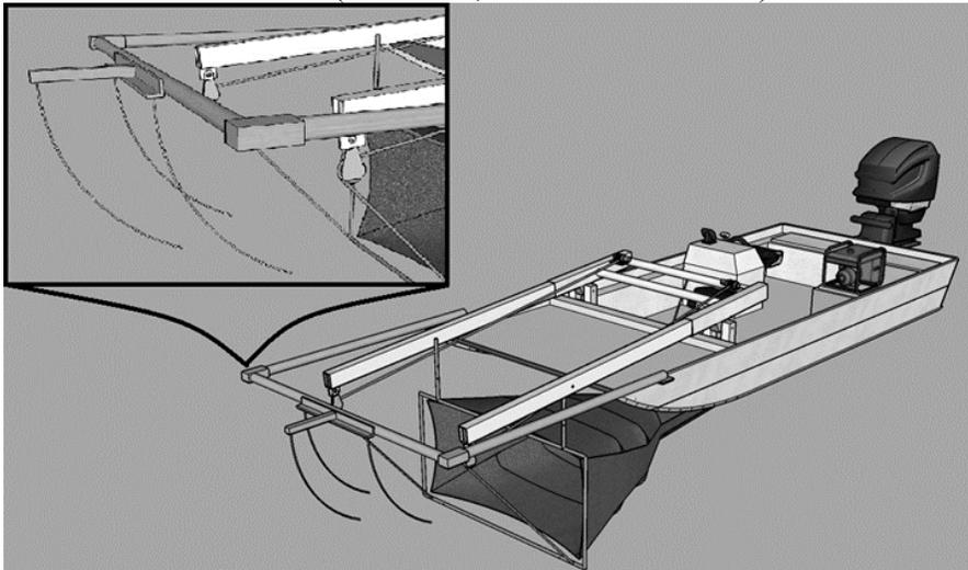
**Figure 3.** *Generalized schematic of the electrified dozer trawl.*
