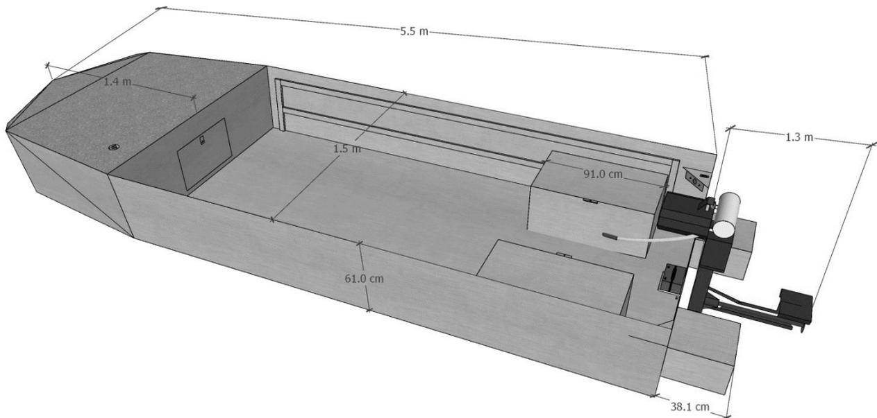
**Figure 19.** *Schematic of the shallow drive boat.*
